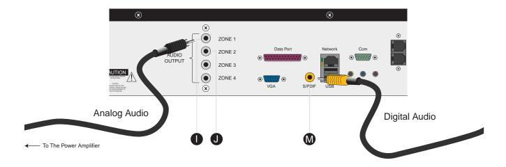
**Digital Audio** – If your equipment supports a digital input, connect an audio cable to the S/PDIF Digital Audio Output **(M)** on the back of the Combo player. Connect the opposite end of the cable to your digital sound equipment. ONLY CONNECT THE ANALOG OR DIGITAL CABLE. NOT BOTH.
